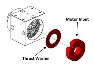
**Step 3**: Attach the Motor Input Block to the NeveRest Motor (with previously attached pinion) using the included M3-0.5 Socket Head Screws and lock washers. Be sure to install the Motor Input Block with the flat side against the motor.
