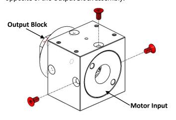
**Step 2**: Remove the Motor Input Block and the steel Thrust Washer. Set the Thrust Washer aside on a clean shop towel or paper towel.
