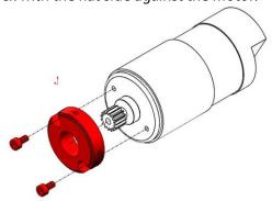
**Step 4**: Reinstall the Thrust Washer into the NeveRest Sport onto the surface of the gears inside the gearbox. Insert the Motor Assembly into the gearbox, and gently turn the output shaft until the gears mesh.
