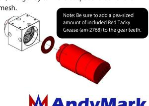
**Step 5**: Align the tapped holes on the circumference of the Motor Input Block and reinstall the M3 flat head screws to secure the Motor Assembly.
